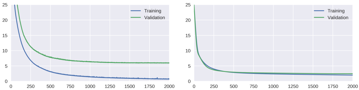
Figure 3.9: Examples of a model that is overfitting (left) and one that is not (right).
